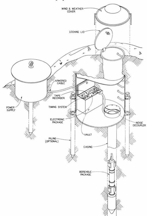
UNMANNED SEISMIC OBSERVATORY as designed by Division 9233 is shown in a typical underground installation. Borehole package is positioned inside the pipe by a gyro unit and mechanically locked in place. Center section of the package rotates to align short period seismometers to compass points. Long period seismometers are in lower section with stabilizing weight.
